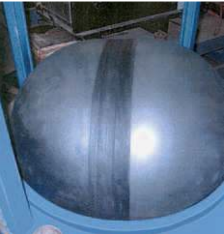
Testing of multi axial strain according to ASTM D5617, on Elastoseal membrane and Thermobond seam.
